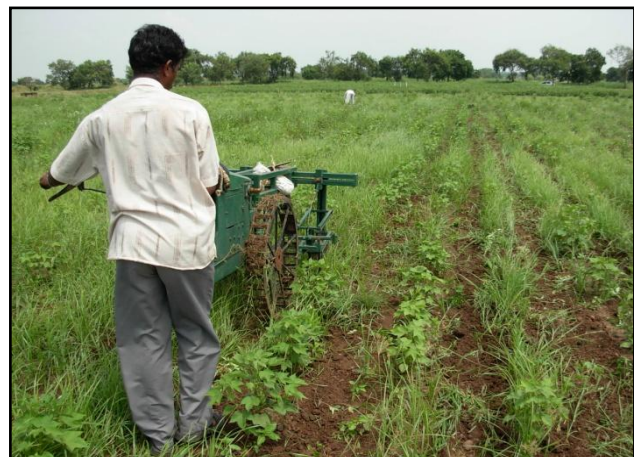
Plate1: Self Propelled Inter Row Cultivator in Operation
