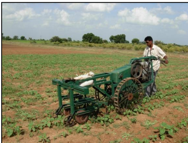
Plate1: Self Propelled Inter Row Cultivator in Operation
